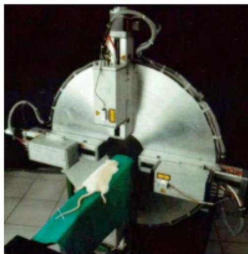
Fig. 21 - PET de elevada resolução para pequenos animais. ([http://technologytransfer.web.cern.ch/TechnologyTransfer/Objects/TT/technologies/SmallAnimalPET\\_small.jpg](http://technologytransfer.web.cern.ch/TechnologyTransfer/Objects/TT/technologies/SmallAnimalPET_small.jpg))
